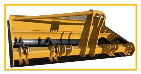
This float is designed for construction and asphalt paving. It is the best to use on hard ground. The vertical back on the drag helps roll larger rocks in front of it instead of riding over the top of them. The back can be used to push for back filling trenches and holes. This float has four USA made ripper shanks that manually fold down and are ready to use. Our customers use these implements in heavy construction settings, and they are built to last.
